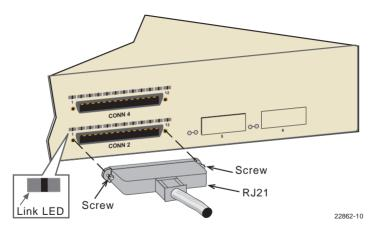
Figure 3-6 Straight Cable Connection
